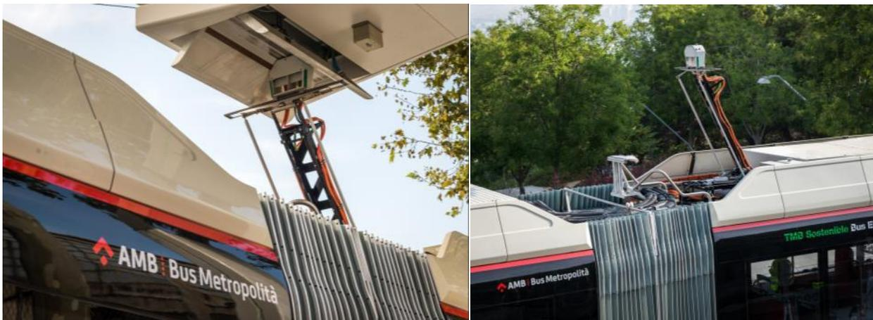
The pantograph connects to the top part of the rapid charge station
